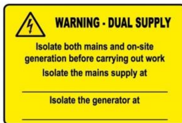
Figure 20 - Warning with a specification of the dual power supply
